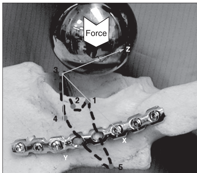
Fig. 6. We arbitrarily assigned 5 points to the acetabulum. Motion was greatest at point 3; thus, we chose this point as the origin of the axes. We defined the x axis with respect to the edge of the anterior and posterior walls of the acetabulum. We determined the y axis by the fracture plane and drew it perpendicular to the x axis. We determined the z axis by the right hand rule.
