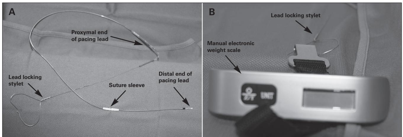
**Fig. 4.** (A) Lead locking stylet connected to the pacing lead to allow attachment of the manual electronic weight scale. (B) Manual weight scale attached to the back of the lead locking stylet.
